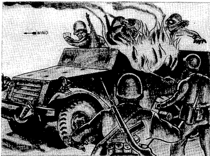
FIGURE 26.—Do not remain in vehicle during burning-off process. Dismount and go up wind.
